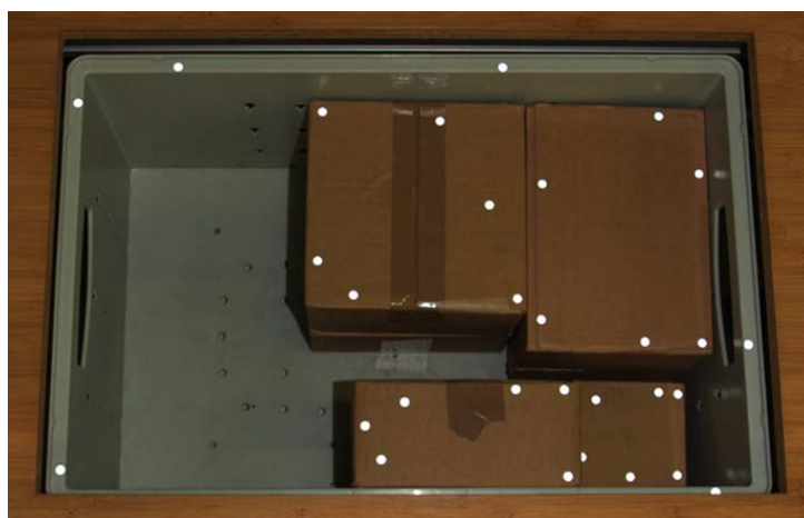
Figure 12: Container status after the placement of 6 boxes. The 7th box (Box016) can not be fit in the “bottom-left” corner (the largest free area in the container) in the orientation it arrives at the infeed conveyor. Therefore, it is flipped and fitted in such a corner.
