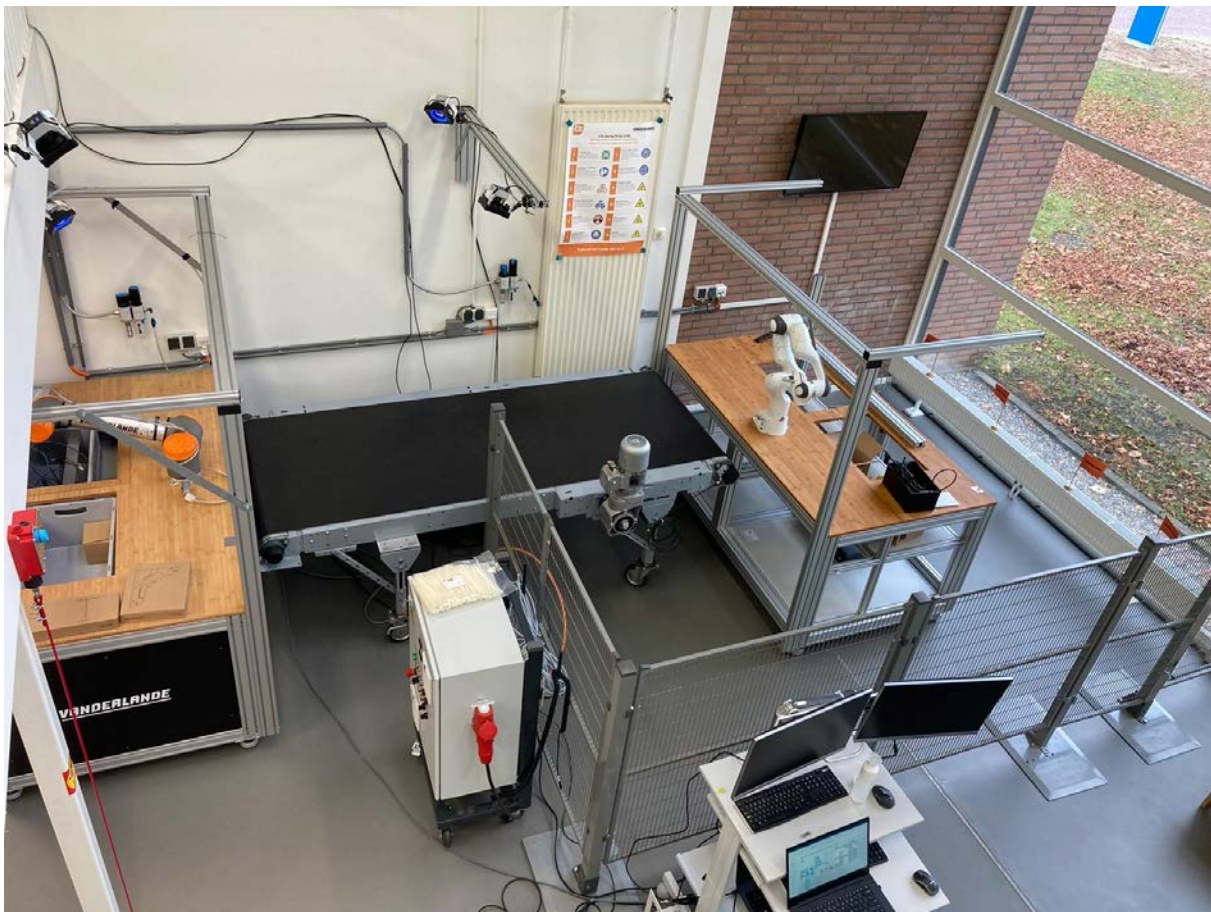
Figure 14: The test setup used for the validation of the TOSS scenario with the workspace of the UR on the left, the belt in the middle and the work space of the Franka Emika robot on the right
