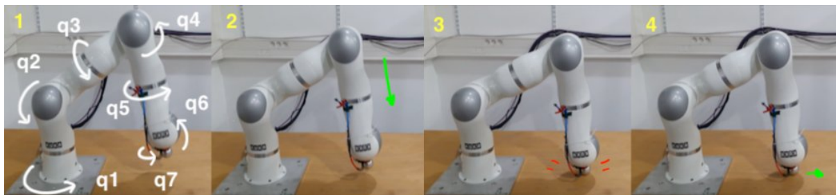
Figure 4: Example of a vertical impact test at 0.2 m/s conducted on a KUKA LWR IV+ robotic arm. The figure shows four snapshots from a recorded video. Time evolves from left to right and from top to bottom. Starting from a rest pose (1), also illustrating the robot 7 DoFs, the robot moves down (2). After impact (3), the end-effector slides on the table (4), keeping contact. Image taken from [10].
