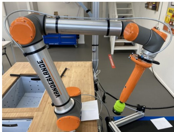
Figure 9: Photo of the robot configuration, showing the robot arm (UR10), the custom suction gripper and the tool changer
