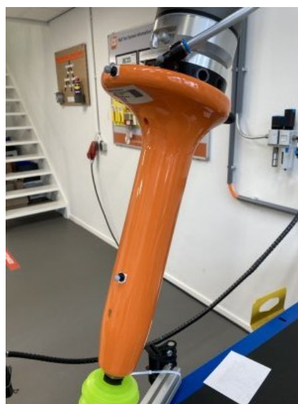
Figure 11: Photo of the tool arm, located between the tool changer and the end effector.
