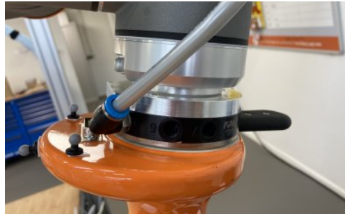
Figure 10: Photo of the tool changer, mounted between the tool arm and the UR10.
