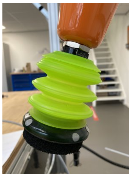
Figure 12: Photo of the end effector, mounted to the tool arm.
